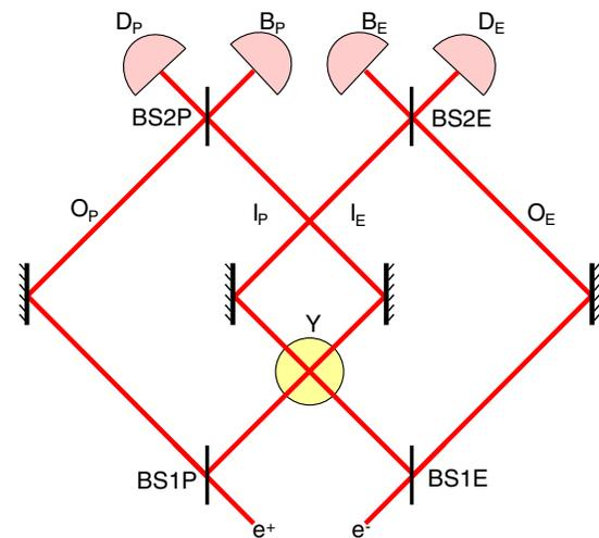
FIG. 1 (color online). Hardy's paradox setup.  $E$  and  $P$  indicate electron and positron, respectively, which can collide in region  $Y$ . BS1P, BS1E, BS2P, and BS2E are 50:50 beam splitters.  $D$  and  $B$  are the dark and bright ports of the interferometers, respectively.  $I$  and  $O$  are the inner and outer interferometer arms, respectively.
