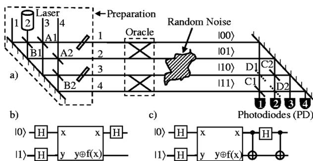
FIG. 1. Schematic of an interferometer which implements the two-qubit Deutsch-Jozsa algorithm (a). All beam splitters are 50/50. With beam splitters  $C1$  and  $C2$  in place, the standard algorithm (b) is performed. We show that an alternate encoding (c) is preferable in the presence of random collective noise on rails 2 and 3; replacing beam splitters  $C1$  and  $C2$  with beam splitters  $D1$  and  $D2$  implements this modified algorithm.
