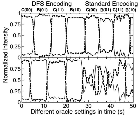
FIG. 4. The probability of the algorithm returning a 0 or a 1 for each of the oracles, in each encoding, with (bottom plot) and without (top plot) the addition of phase noise. The data are extracted by summing the normalized intensities from Fig. 3 for the pair of detectors indicating the constant functions (dashed line), and the balanced functions (solid line). Note that the success rate is close to unity even in the presence of noise when the DFS encoding is used.
