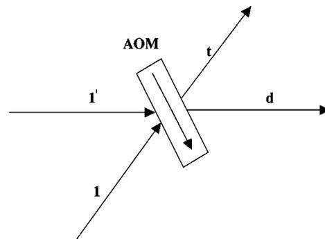
FIG. 1. The two input modes, 1 and 1', enter an AOM and are converted to two output modes,  $t$  and  $d$ .
